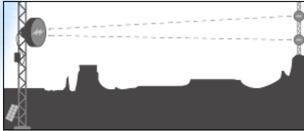
One Dual Pole and Two Single Pole Antennas Vertically Separated
