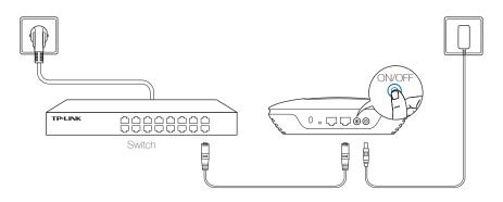
1. Plug one end of the provided power adapter into the POWER port of the EAP and the other end to a standard electrical wall outlet.
