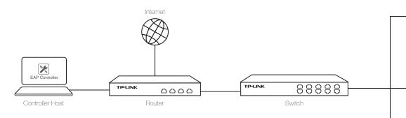
• A DHCP server (typically a router) is required to assign IP addresses to the EAP and clients in your local network
