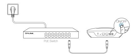
1. Connect the Ethernet cable from the PoE switch to the ETHERNET port.
